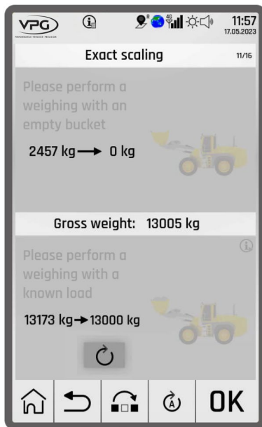
Fig. 8-37: Exact scaling "Span adjustment"
