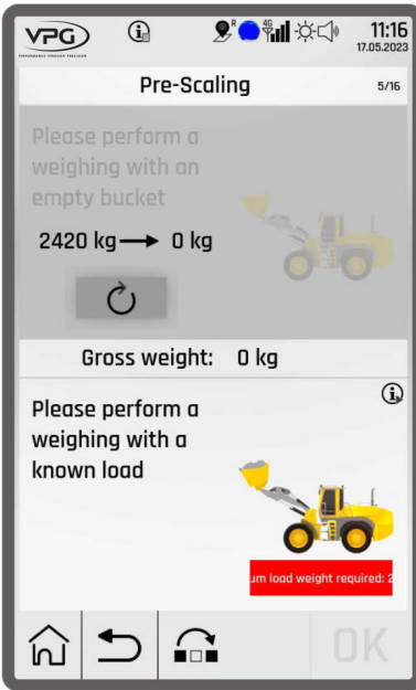
Fig. 8-12: Pre-Scaling – Span Calib. Point
