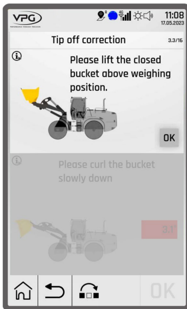
Fig. 8-8: Tip off correction
