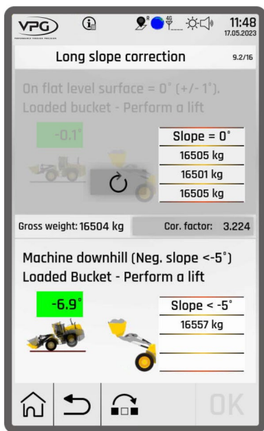
Fig. 8-29: Long slope corr. "Downhill"
