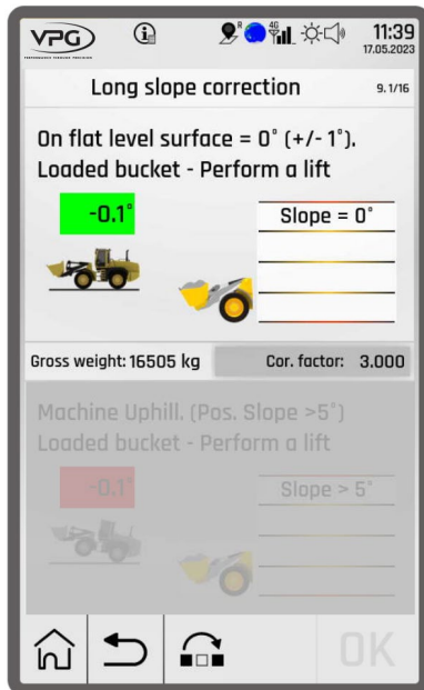
Fig. 8-25: Long slope corr. "Level"
